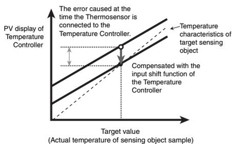
**Gain and Offset Compensation with Two-point Shift Function**
